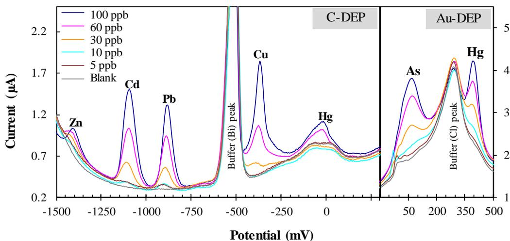
**Figure 3.** Simultaneous electrochemical measurement of six heavy metals in a standard solution using the “DEP-On-Go” system. DP voltammograms are shown for the detection of zinc, cadmium, lead, and copper using a carbon DEP chip (C-DEP), and arsenic and mercury using a gold DEP chip (Au-DEP) in standard solutions. The data are the averages of four to six independent experiments.
