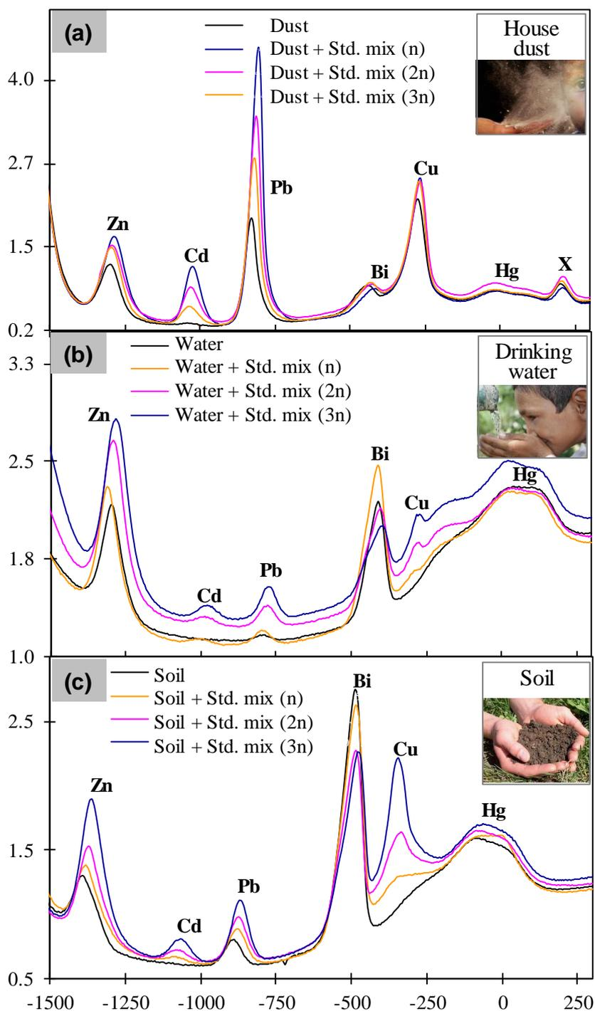
**Figure 4.** Simultaneous electrochemical measurement of various heavy metals in real samples using the “DEP-On-Go” system. DPV curves are shown for the simultaneous detection of zinc, cadmium, lead, copper, and mercury in real samples from house dust (a), drinking groundwater (b), and soil (c). Std. mix = Standard mixture (see Section 2.3).
