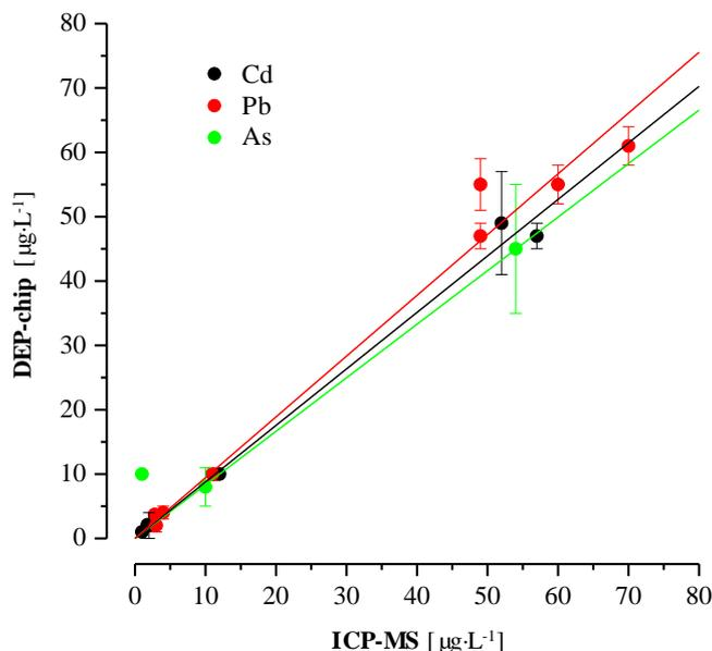
**Figure 5.** A correlation curve between the conventional (ICP-MS) and “DEP-On-Go” device for sensitive detection of cadmium, lead, and arsenic heavy metals in drinking groundwater samples.
