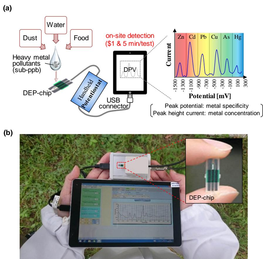
**Figure 1.** “DEP-On-Go sensing” concept. Schematic representation of the work flow (a) and photographs (b) of the sensing platform for the on-site and rapid detection of heavy metal pollutants directly from environmental samples.
